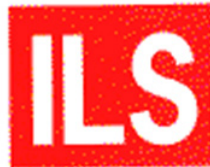
Figure 3.26. ILS Critical Area Holding Position Sign.
