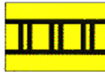
Figure 3.32. ILS Critical Area Boundary Sign.
