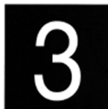
Figure 3.37. Runway Distance Remaining Sign Indicating 3,000 feet of Runway Remaining
