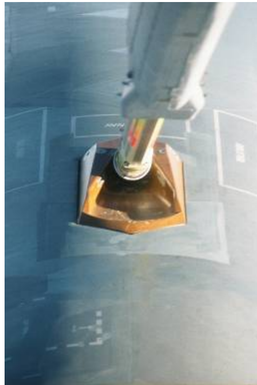
B-2 Receptacle Close-up
