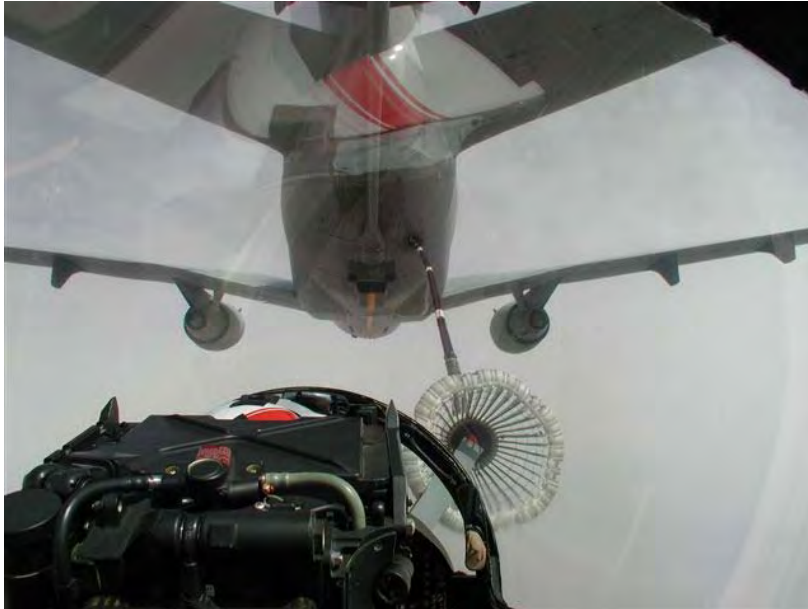
Receiver with probe on right side correctly aligned along tanker centreline
