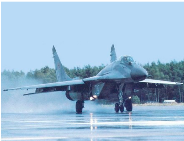
Figure 93: Russian MiG-29 Fulcrum-C. Note the enlarged dorsal spine containing some additional fuel and an internal jammer.
