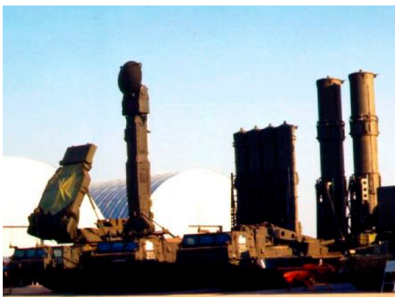
Figure 134: The complete S-300PMU system, consisting (from the left to right) of the 30N6 guidance radar, the 70N6 surveillance radar (mounted on the mast), and the 5P85 launcher vehicles.
