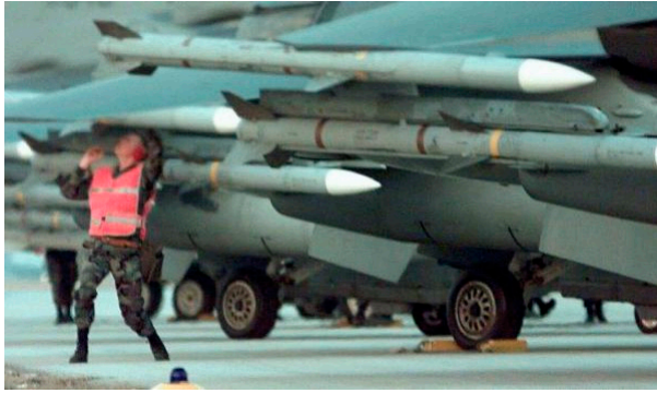
Figure 74: AIM-120C loaded on F-16 wingtip, and AIM-120B on station 8. (Picture credit of USAF)
