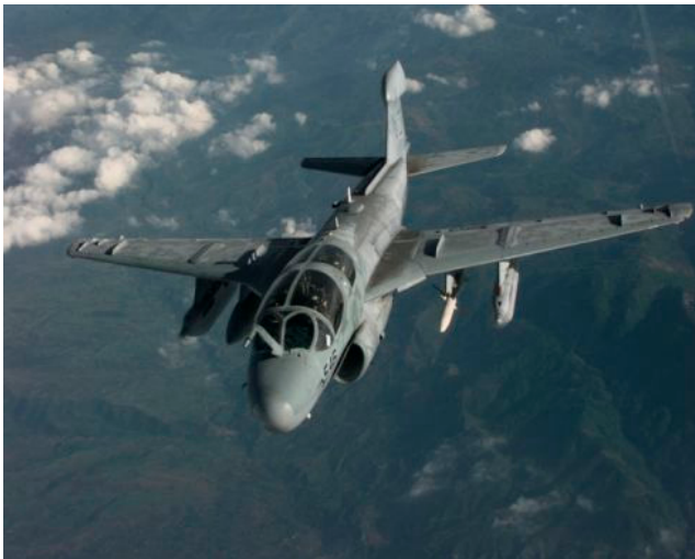
Figure 117: EA-6B Prowler, carrying a mixed load of jammer pods and AGM-88 HARM missile. This is a reflection of the EA-6A's unique combination of lethal and non-lethal SEAD capabilities. (Picture credit of USAF)
