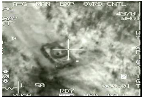
Figure 35: Serbian T-55 caught in the cross hairs of the LANTIRN targeting pod moments before the LGB impact during Operation Allied Force. The LANTIRN targeting pod allows precision strikes to be carried out from medium level altitudes, above the engagement altitude of SHORAD threats. (Picture credit of NATO)
