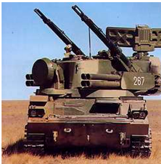
Figure 139: 2S6M anti-aircraft air defense system with twin 30 mm cannons and SA-19 missile system
