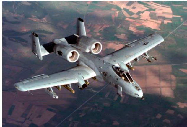
Figure 110: A-10 Thunderbolt II during Operation Allied Force. This airplane carries an ALQ-131 and a pair of AIM-9M for self defense, in addition to the AGM-65D and cluster bombs. (Picture credit of USAF)
