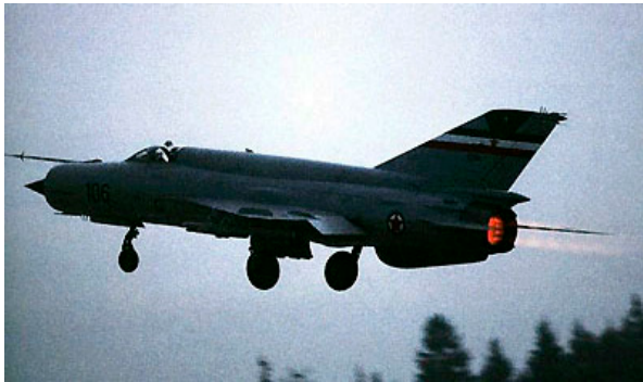
Figure 88: Serbian MiG-21bis taking off. Note the bulged spine on the aircraft compared to the MiG-21PF
