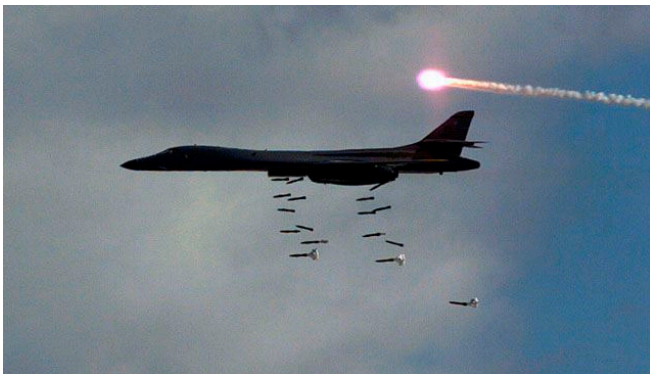
Figure 113: B-1B releasing a stick of BSU-49/B bombs while dispensing flares to defeat IR missiles. (Picture credit of USAF)
