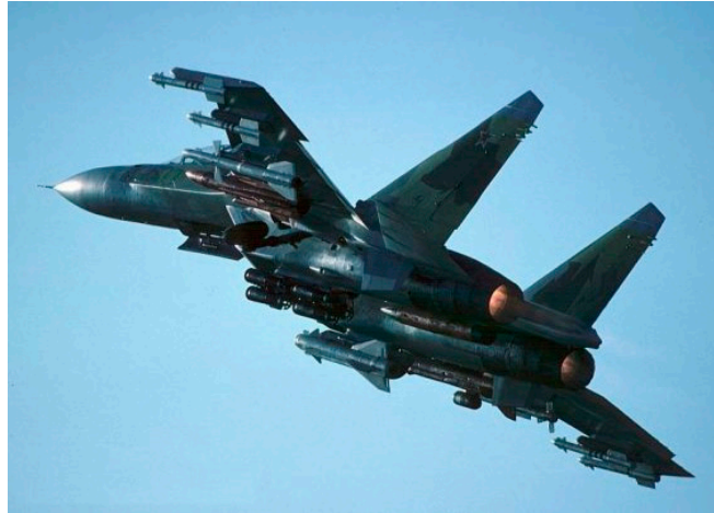
Figure 96: Su-30MKK prototype taking off with a full complement of precision and non-precision air-to-ground ordnance
