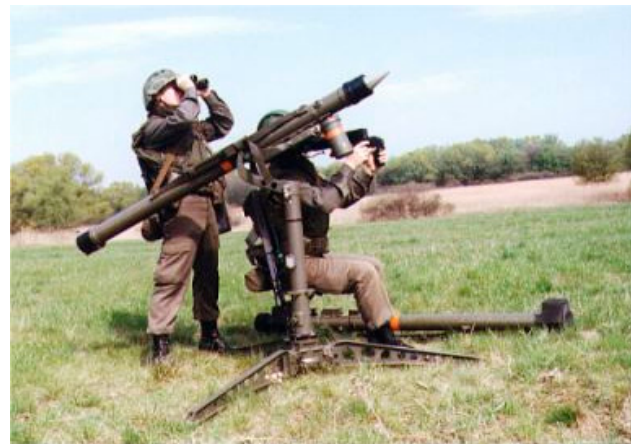
Figure 143: Mistral firing team. Note the unique pyramidal seeker dome.
